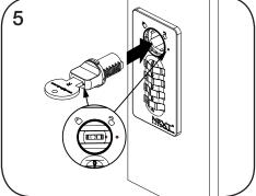
Insert the new Core subassembly into the lock. The triangle mark on the Knob  $\triangleright$  will align with the circle mark O on the face.
