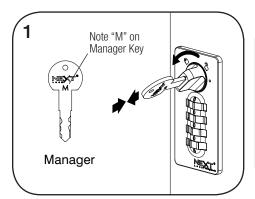
After opening the door with the Manager Key, leave the door open and use the Manager Key to turn the knob to the "Locked" position. Remove the Manager Key.
