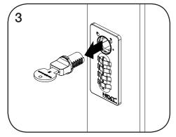
Pull the Removal Key to remove the old Knob and Core.
