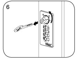
Turn the knob to the unlocked  $\ \Box$  position. Remove the Replacement Removal Key.
