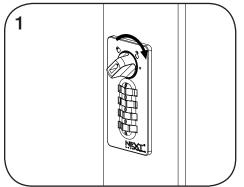
Turn the knob to the unlocked D position.
