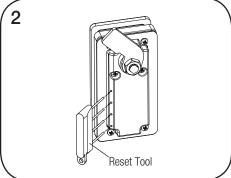
Insert the Reset Tool into the four pin holes on the rear of the unit.
