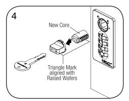
Insert the replacement Removal Key into the old Knob and place the NEW Core on the Knob. The triangle mark ▶ on the knob should be aligned with the Raised Wafers.
