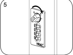
Remove the Reset Tool and turn the knob to the unlocked  $\ensuremath{^{\square}}$  position.
