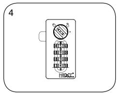
The final code displayed is the current code. In this example, the combination was 5-9-9-4.
